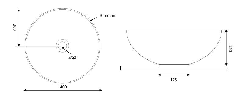
Sizes detailed could have a variation of about +/-5 % due to the changes to material characteristics during the firing processes. Exact measurements for individual installations can only be taken from the finished ceramic
